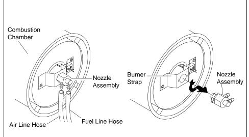
Figure 9 - Removing Air and Fuel Line Figure 10 - Removing Nozzle Assembly Hoses
